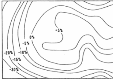
Fig. 12. Background light distribution over the screen.
