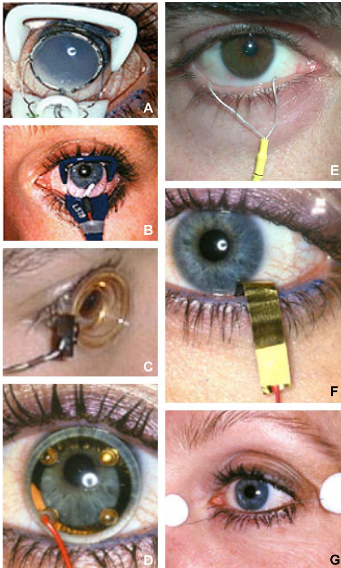
Fig. 1. Standard recording electrodes for ERG tests: (A–D) corneal electrodes; (E–G) conjunctival electrodes (pictures adapted from Refs. [2,3]).
